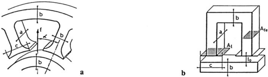
Fig. 13 Single U-shaped electromagnet as part of a radial bearing a) real geometry b) simplified geometry
